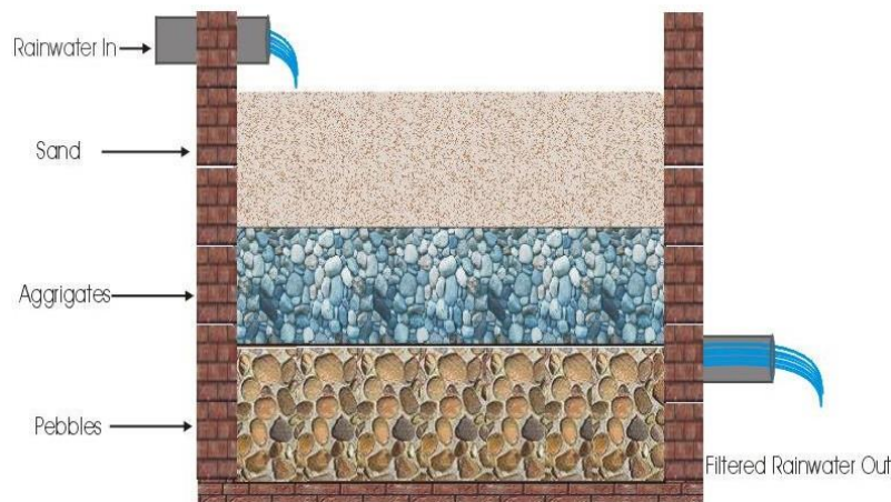
Figure No. 3 Design of Rainwater harvesting pit
